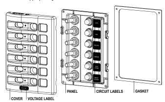
Securely tighten switch and circuit breaker boots.
